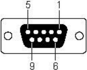
The diagram shows a DB9 connector with a 9-pin D-subminiature connector. The pins are arranged in a 3x3 grid. Pin 1 is at the top right, pin 5 is at the top left, pin 9 is at the bottom left, and pin 6 is at the bottom right. The connector is shown in a perspective view with two mounting holes on the sides.
