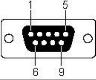
The diagram shows a 9-pin D-sub connector. The pins are arranged in a 3x3 grid. Pin 1 is at the top left, pin 5 is at the top right, pin 6 is at the bottom left, and pin 9 is at the bottom right. The connector is shown in a perspective view with two mounting holes on the sides.
